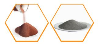
The properties of some Cu-based alloys have become important options, while others have been mainstays of the diamond tooling industry. Overall Cu alloy powders are better as a metal bond for diamond tools and also have good properties in the fabrication of diamond tools
